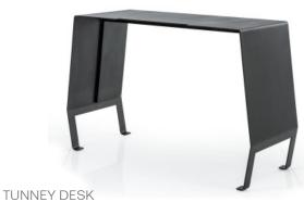
The Tunney Desk is fabricated from a single sheet of steel that has been folded to create integral legs. A rear recess for cord management is also incorporated into the fold. 3/16" plate steel with matte, blackened finish. W 48" x D 18" x H 30"
